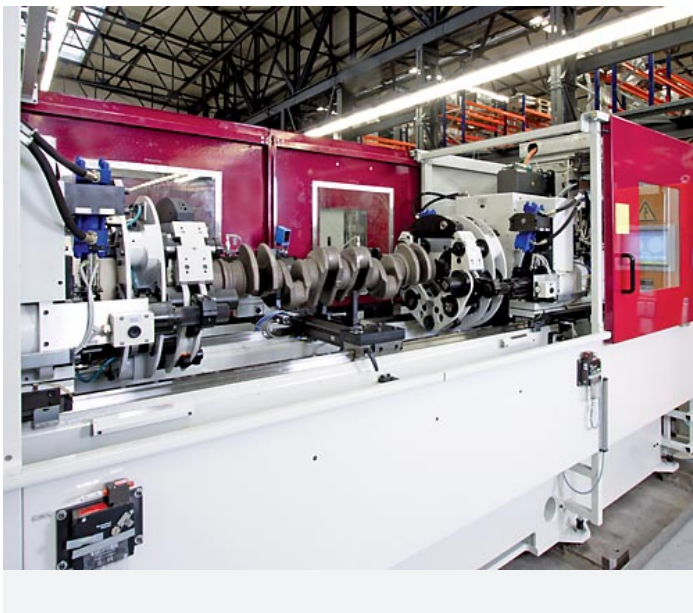
Mass-centering machines for vehicle crankshafts; high flexibility through sledge construction
