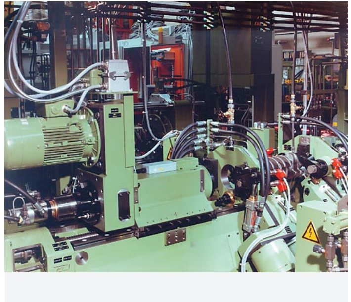
Drill units with hydraulic or electro-mechanical feed for drilling the center holes. Adjustable to various crankshaft lengths. Precision drill spindles for high centering accuracy. In the case of a separate centering station the crankshaft is clamped at the main journals and restrained by means of alignment elements. Adjustment to the optimum centering position is achieved by positioning motors, numerically controlled from the measuring equipment.
