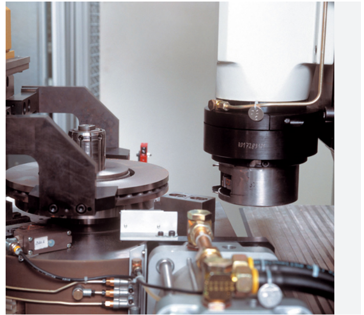
Multi-station machine for balancing of brake discs, with lift-and-turn transfer device. The initial unbalance is determined in the measuring station and then corrected in the correction station, following which the residual unbalance is checked. Performing these processes on separate stations optimizes cycle time.
